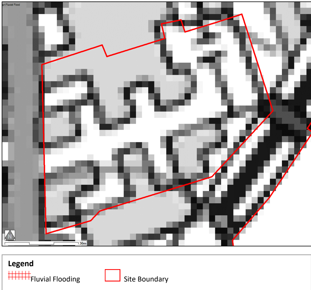
Figure 10 Fluvial Flooding ( 1 in 100 year + 17%CC)
