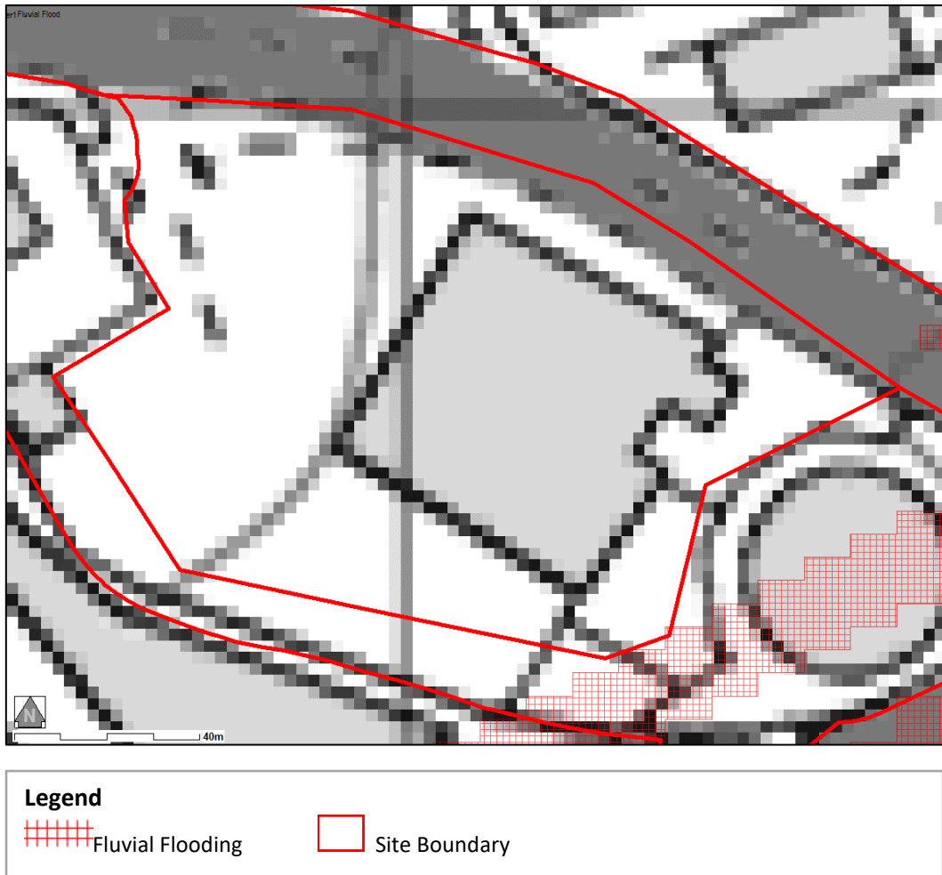
Figure 10 Fluvial Flooding ( 1 in 100 year + 17%CC)
