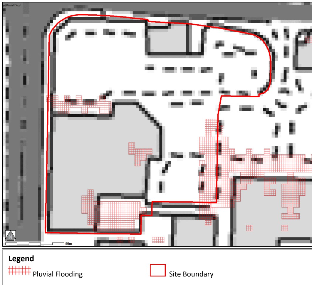
Figure 12 Pluvial Flooding (1 in 100 year + 17%CC)
