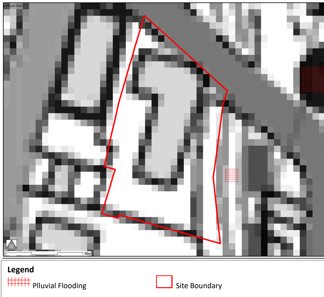
Figure 12 Pluvial Flooding (1 in 100 year + 17%CC)
