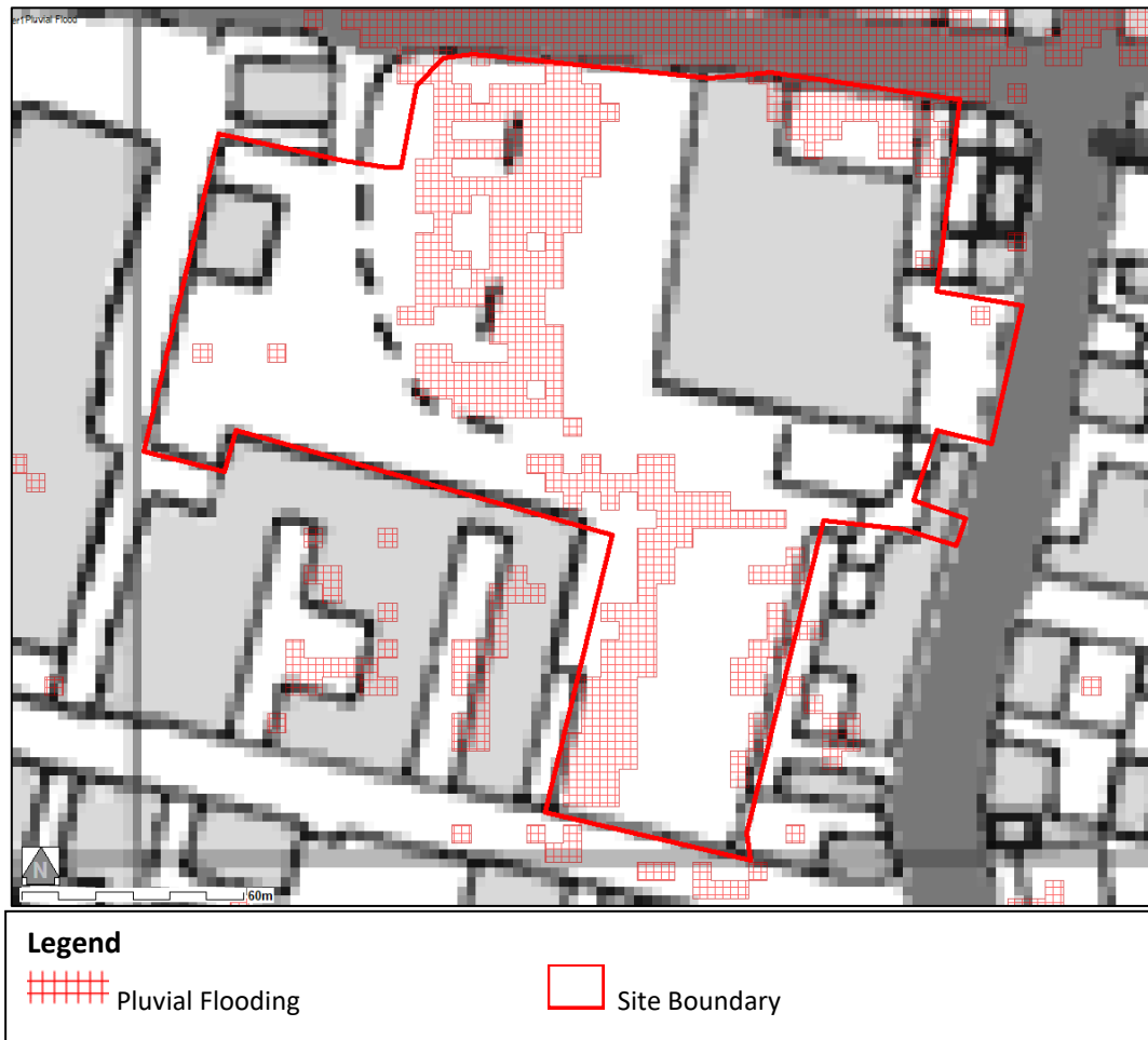
Figure 12 Pluvial Flooding (1 in 100 year + 17%CC)
