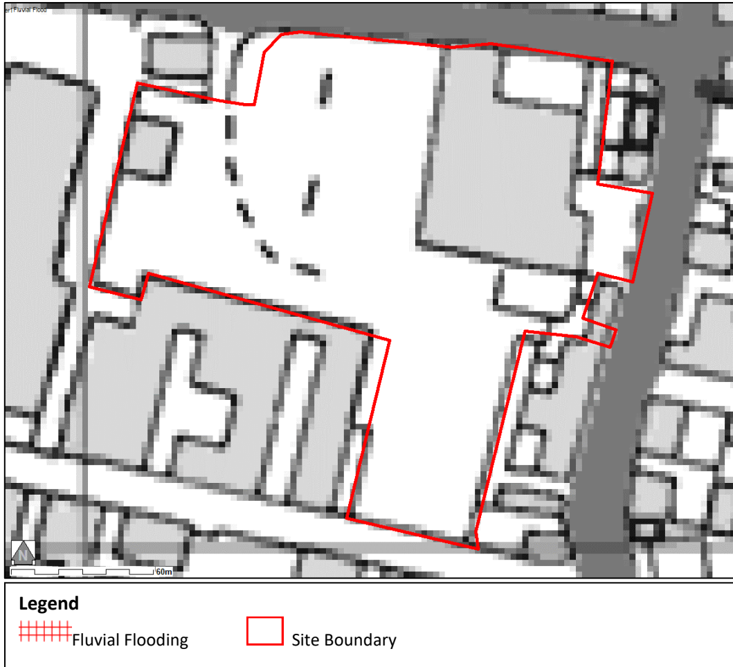
Figure 10 Fluvial Flooding ( 1 in 100 year + 17%CC)
