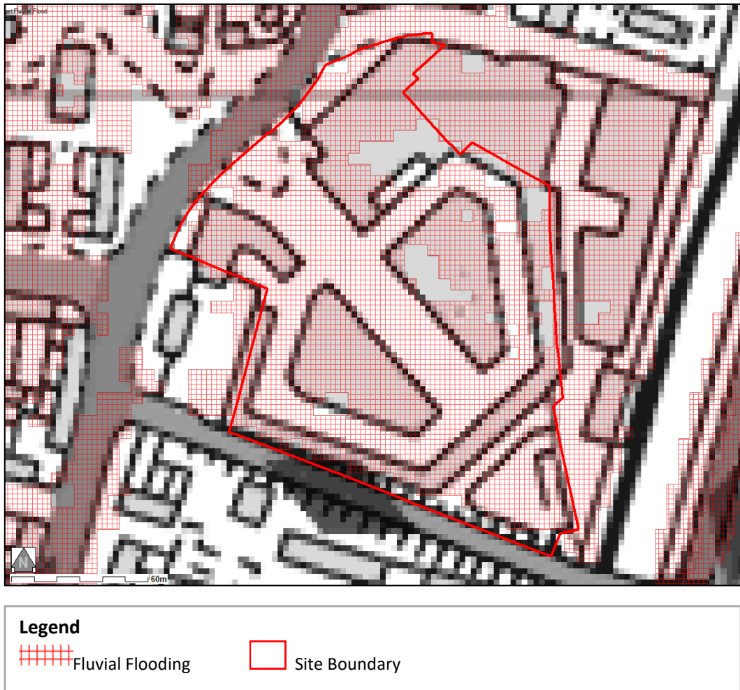
Figure 10 Fluvial Flooding ( 1 in 100 year + 17%CC)
