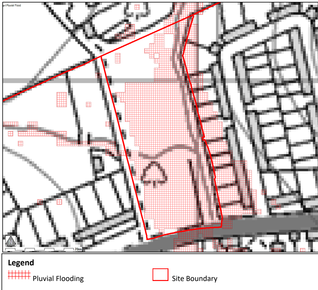
Figure 12 Pluvial Flooding (1 in 100 year + 17%CC)
