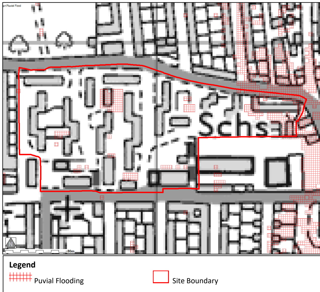
Figure 12 Pluvial Flooding (1 in 100 year + 17%CC)
