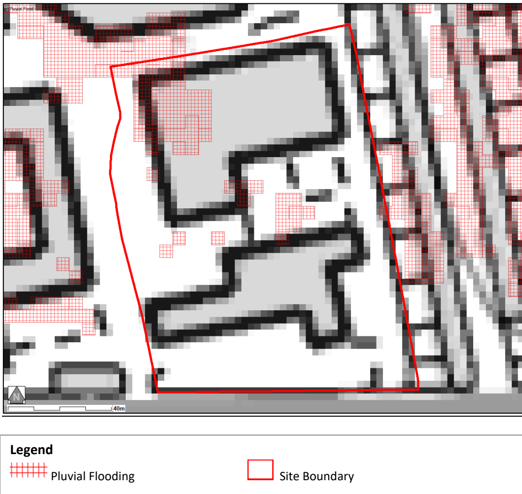
Figure 12 Pluvial Flooding (1 in 100 year + 17%CC)
