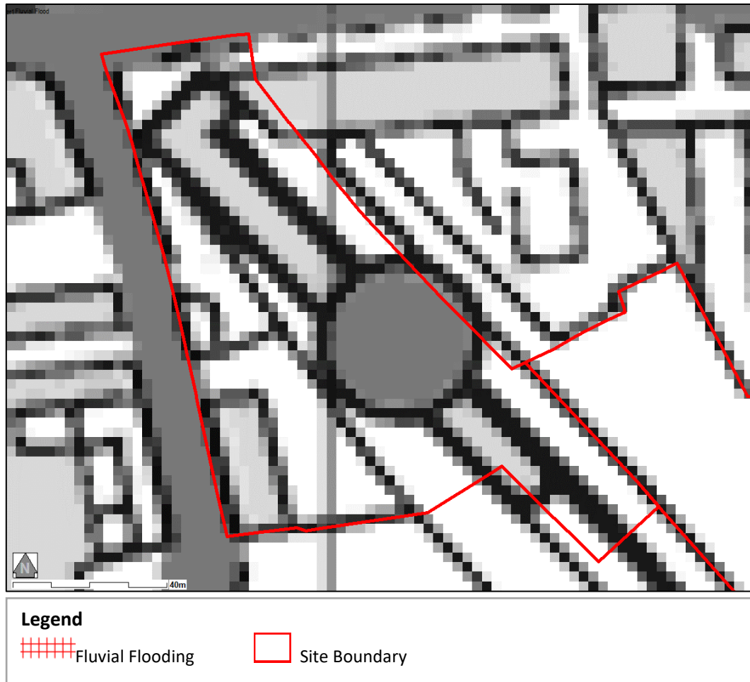
Figure 10 Fluvial Flooding ( 1 in 100 year + 17%CC)
