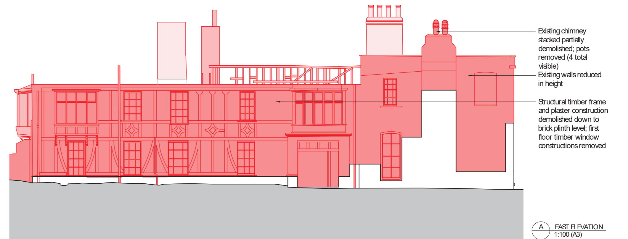
Above: Proposed demolitions and retentions of the west elevation of Broomfield Park House
