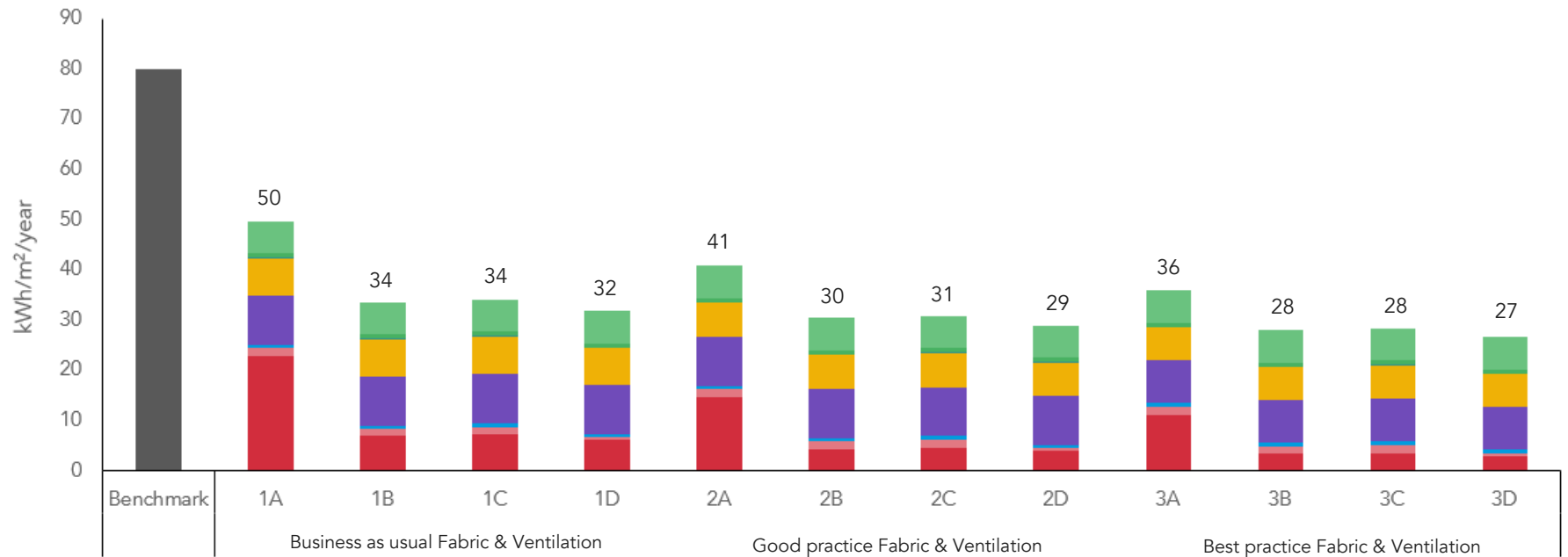
Figure 7.7 - Predictive energy modelling results: bar chart showing the detailed breakdown of energy use intensity (EUI) for each case
