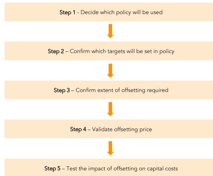
Figure 10.7 - The above process is recommended to estimate the additional cost of offsetting.
