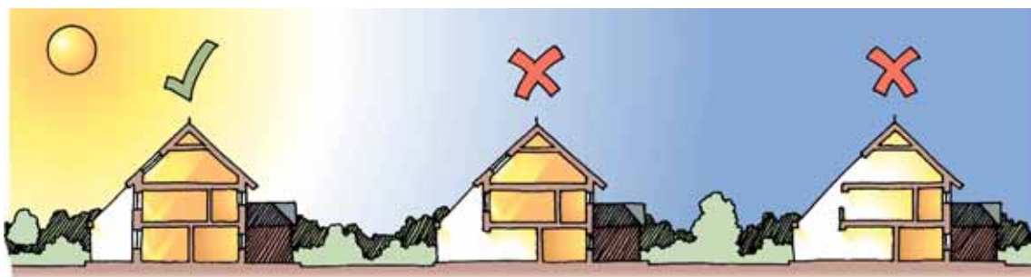
Figure 1: Conservatories and sunspaces should be separated from the main building to reduce heat loss and improve performance
